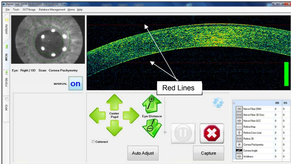
**Figure 31 Use Distance Arrows to Place Cornea Image between Red Lines**
