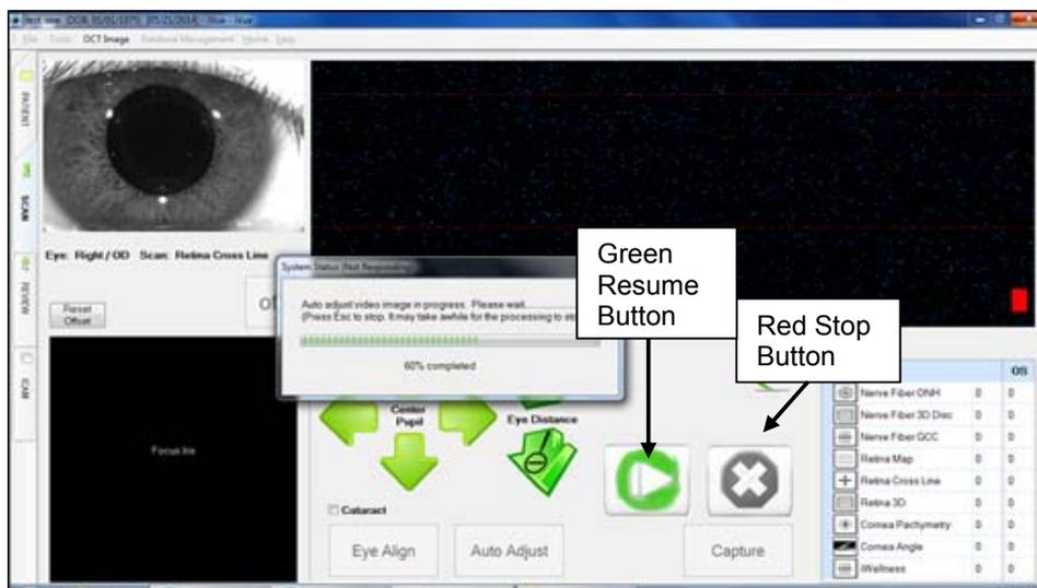
**Figure 25 System Paused, Green Resume Button Visible**
