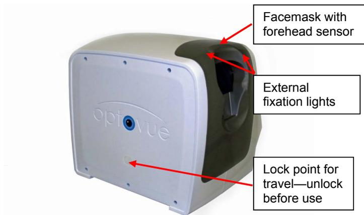
**Figure 2 System Rear View**
