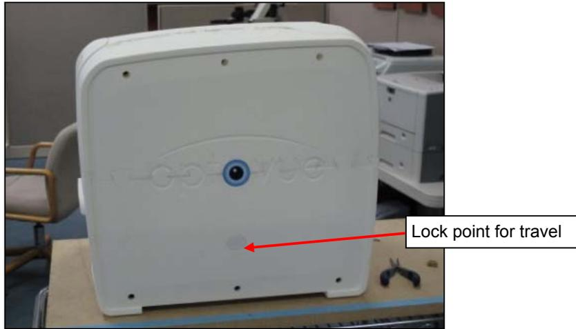
**Figure 3 Lock Base Before Moving System**
