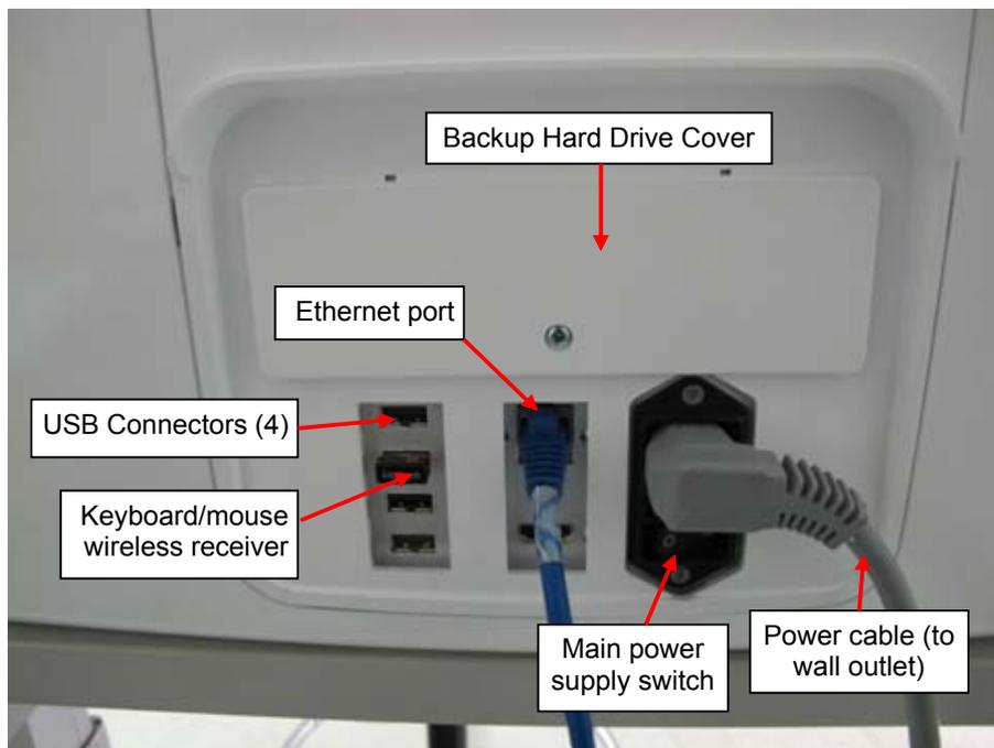
**Figure 4 Connectors on Right Side**
