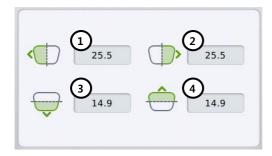
You can modify the lens shape by entering the values directly in the Input Area.
