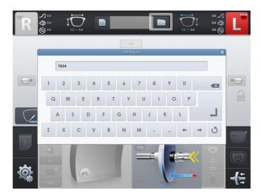
The function of job request works only when communication option on configuration menu is set properly.
