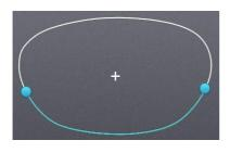
Set modification area by touching any point on lens shape. The point becomes the center of the modification area. To adjust modification range, touch and drag one of 2 touch points around the selected lens shape (blue).
