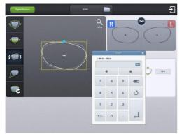
After selecting the item to change, enter the value using the numeric keypad.
