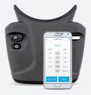
Self-test refraction tool powered by a smartphone.
