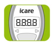
Following a brief pause, the display will show "LoAd," reminding the user to load the single use probe into the tonometer prior to measurement.
