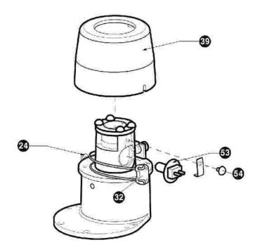
[Figure 8. Replace Halogen bulb]
