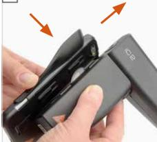
Attach the mobile phone case to the HEINE iC2 by sliding it upwards until it engages.
