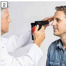
**2** Start the app and activate the image capture mode, push the trigger button on the device, the light has to be on. Position the device with a distance of approx. 10 cm to the patient's eye and monitor the eye to be examined on the display. A red reflex should be visible already. Approach the eye slowly until approx. 3 cm until fundus structures are identifiable on the display. The left hand stabilizes the instrument at the patient's head and may lift the upper eyelid.
