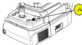
9-3. For enhancing OCT signal, move position of reference mirror by pressing arrow of REF.M icon
