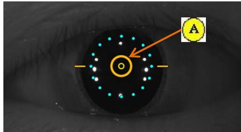
8-4. If auto tracking is on, alignment and focus is automatically accomplished in tracking region.
